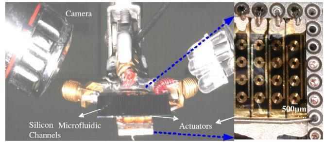
FIG. 4. (Color online). The spacer aligned on top of the  $4 \times 4$  ejector array with silicon micromachined microfluidics channels that control fluid level.
