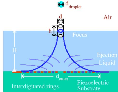
FIG. 3. (Color online). The cylindrical acoustic focus at the surface of the fluid.
