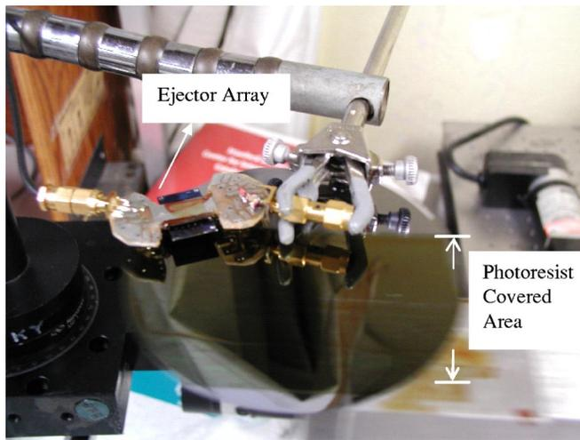
FIG. 9. (Color online). Full photoresist coverage of a 4 in. wafer with  $2.4\ \mu\text{m}$  thick photoresist.
