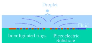
FIG. 2. (Color online). Physical operation of a fluid loaded 2D ejector array (side view).
