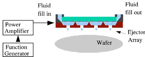
FIG. 6. (Color online). Block diagram of the photoresist deposition setup.
