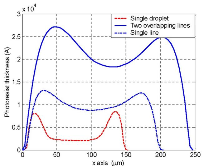
FIG. 8. (Color online). Photoresist single drop, single line, and two overlapping line profiles on the wafer surface of two simultaneously ejected overlapping lines.
