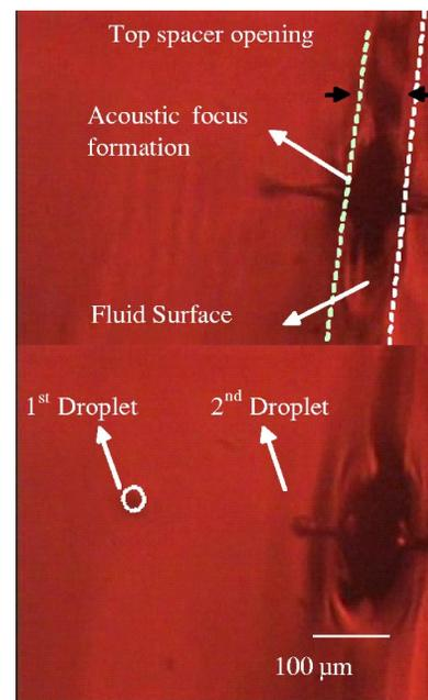
FIG. 5. (Color online). Ejected  $21 \mu\text{m}$  diam photoresist solvent droplets from a  $100 \mu\text{m}$  wide spacer opening.
