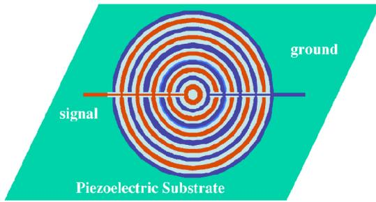
FIG. 1. (Color online). Geometry of the 2D ejector array (top view).
