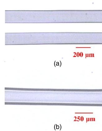
FIG. 7. (Color online). Two simultaneously written photoresist lines on wafer surface; (a) separated and (b) overlapping by  $150\ \mu\text{m}$  in order to write a wider  $250\ \mu\text{m}$  wide line.
