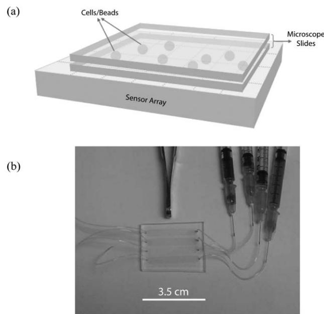
**Fig. 1** (a) A simplified sketch of LUCAS. Cells to be imaged are illuminated by a collimated light source, and the shadow of each cell is recorded by an opto-electronic sensor array (*e.g.*, a CCD chip) without using any lenses. (b) A four channel microfluidic device that can be integrated with the LUCAS system. Such channels could be functionalized and used to selectively capture *e.g.*, CD4 cells from whole blood. LUCAS can monitor all 4 microfluidic channels simultaneously.
