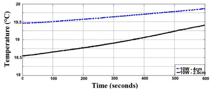
Fig. 10. Temperature increment in the depth of 2.5 cm and 4 cm with 10 W input power.
