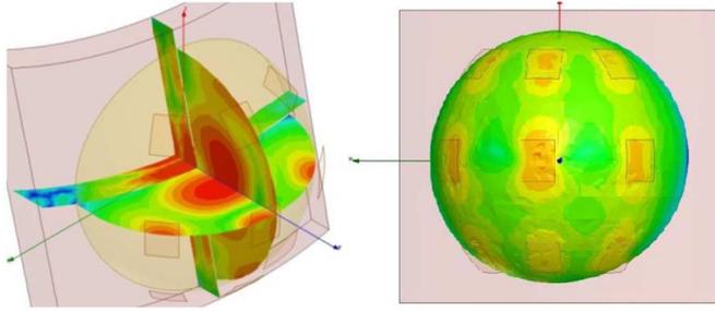
Fig. 2. Simulation of SAR distribution in the breast model.
