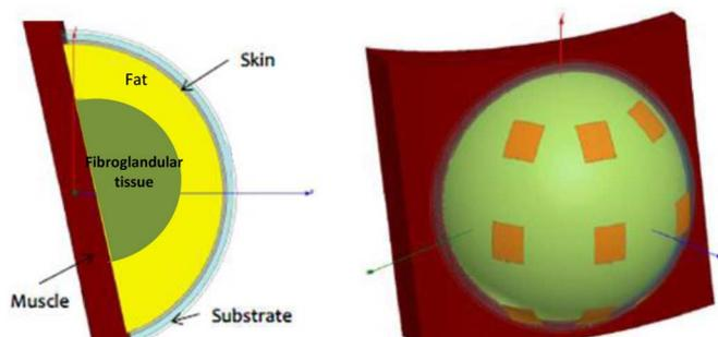
Fig. 1. Simplified breast model for simulations (Ansys HFSS). Breast geometry (left), Microwave antenna applicator on the model (right).
