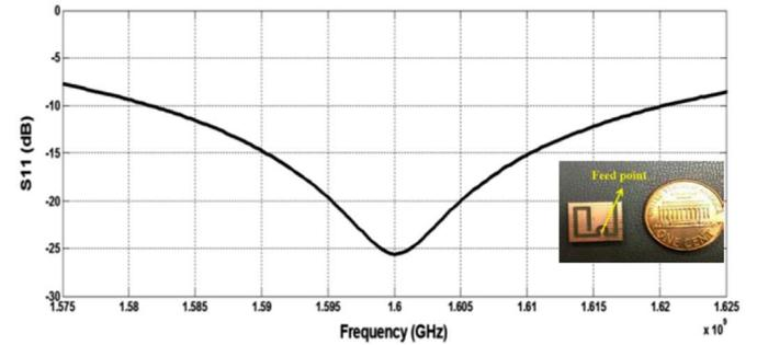
Fig. 5. Return loss of the MW antenna.
