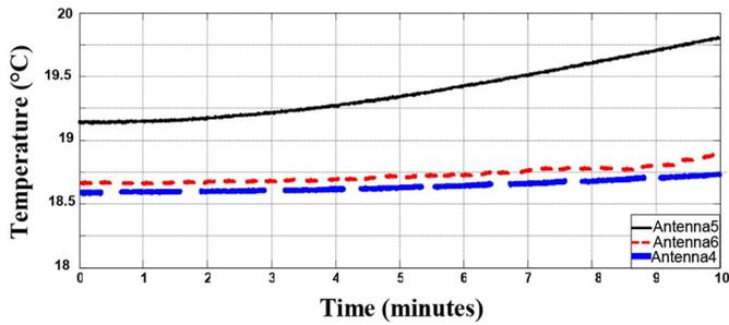
Fig. 11. Temperature increment in the depth of 2.5 cm at 1.6 GHz with 5 W input power.
