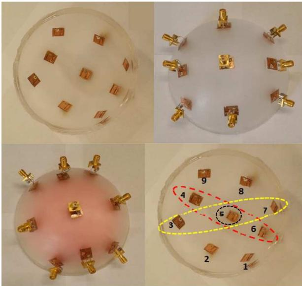
Fig. 6. Microwave antenna applicator printed on a flexible material and the combination of fed antenna during the measurements.
