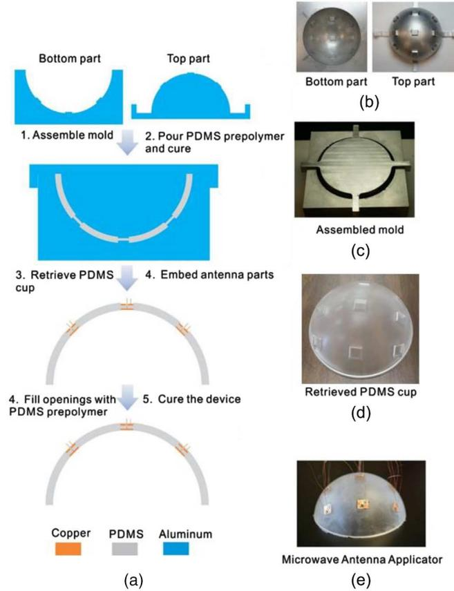
Fig. 3. Fabrication procedure of flexible microwave antenna applicator. (a) Schematics of fabrication. (b) Top and bottom parts of the aluminum mold. (c) Assembled mold. (d) Retrieved PDMS cup. (e) Final microwave antenna applicator.
