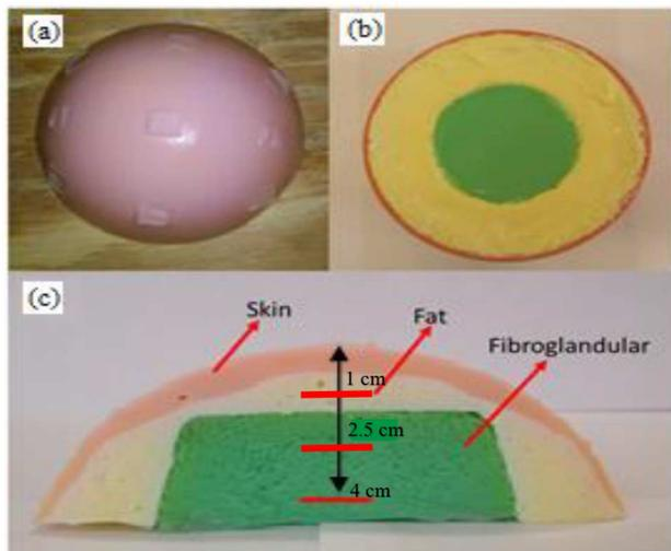
Fig. 7. (a) Top view, (b) bottom view, and (c) cross section of the breast mimicking gel.
