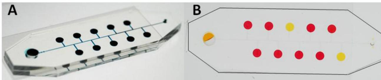
**Fig. 6. Autonomous microfluidic device for the measurement of MIC of antibiotics against bacterial pathogens**
