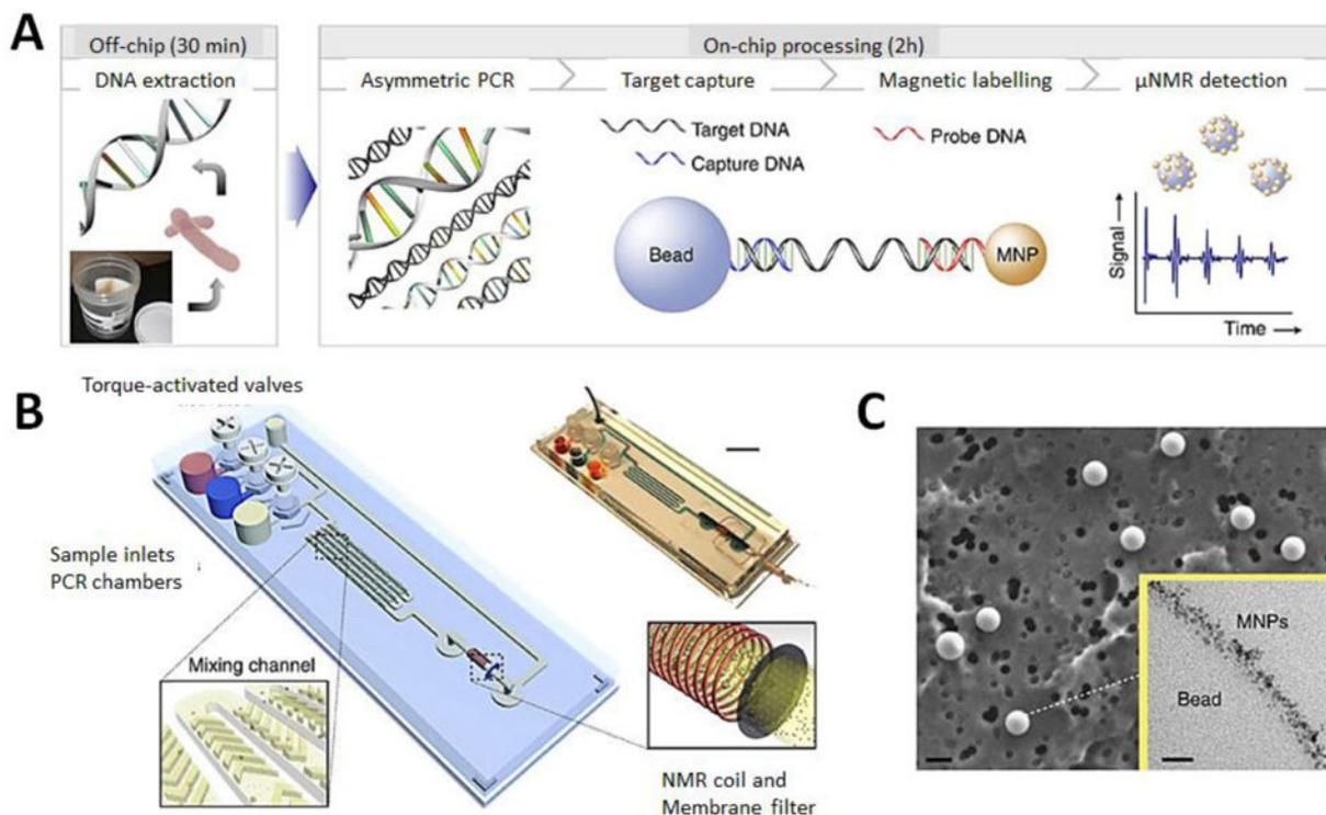
**Fig. 2.  $\mu$ NMR fluidic chip that enables the detection of Mtb target DNA from sputum using a magnetic biobarcode approach**
