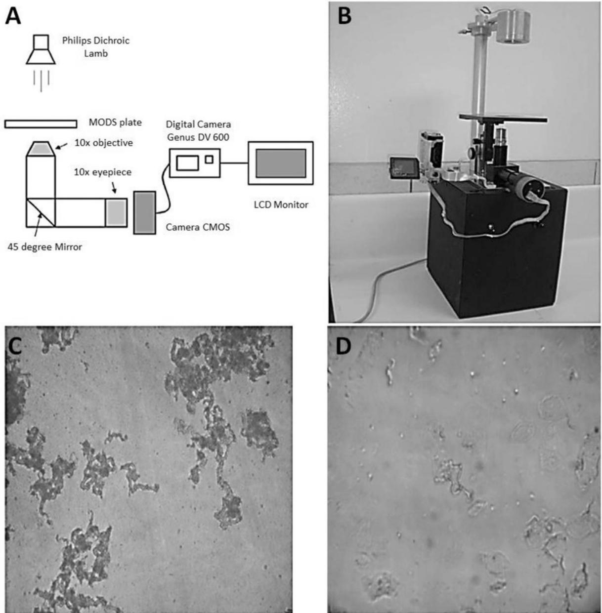
**Fig. 4. A mobile platform for detection of whole Mtb bacteria**
